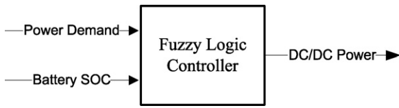
Fig. 8. Fuzzy logic controller for power split.
